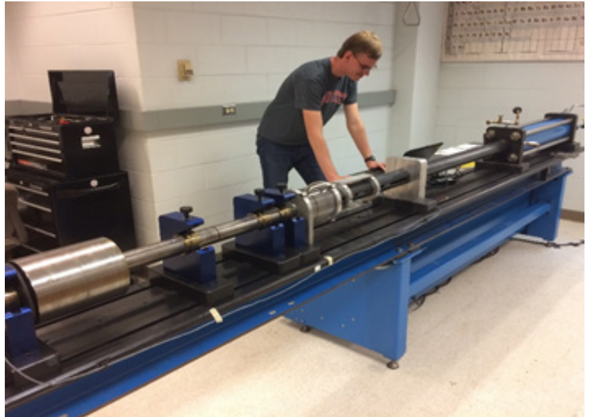
Grad student Mike Braunagel setting up an experiment on the Split Hopkinson Pressure Bar apparatus in the OSU Structural Geology & Geomechanics Lab
