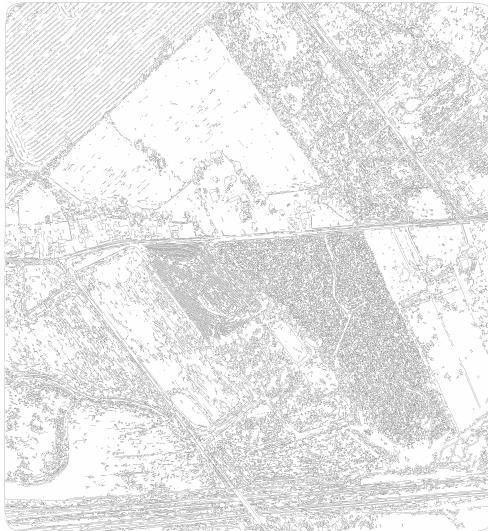
Figure 2.6 Edge detection at refined resolution ( S = 1.6 , width = 23)
