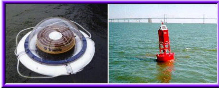
Figure 3.1: A waverider buoy (left, a floater design). An autonomous spar buoy (right) used by NOAA/NGS in San Francisco Bay (Zilkoski et al., 1996).
