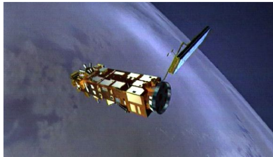
Figure 4.4. Artist's impression of ENVISAT after the completion of the primary deployment of the solar arrays. (Courtesy of ESA).
