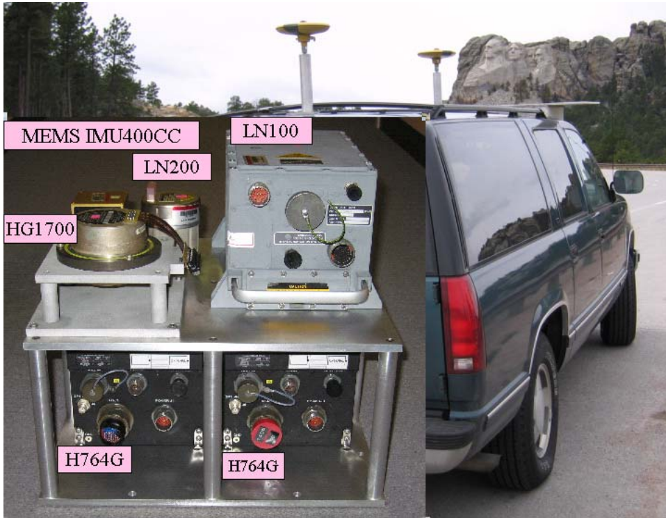
Figure 2.4. OSU GPS/INS AIMS™ hardware configuration.
