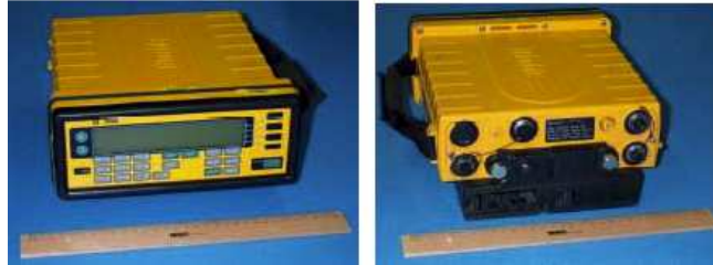
Figure 3.2: Trimble 4000SSE front and rear view.
