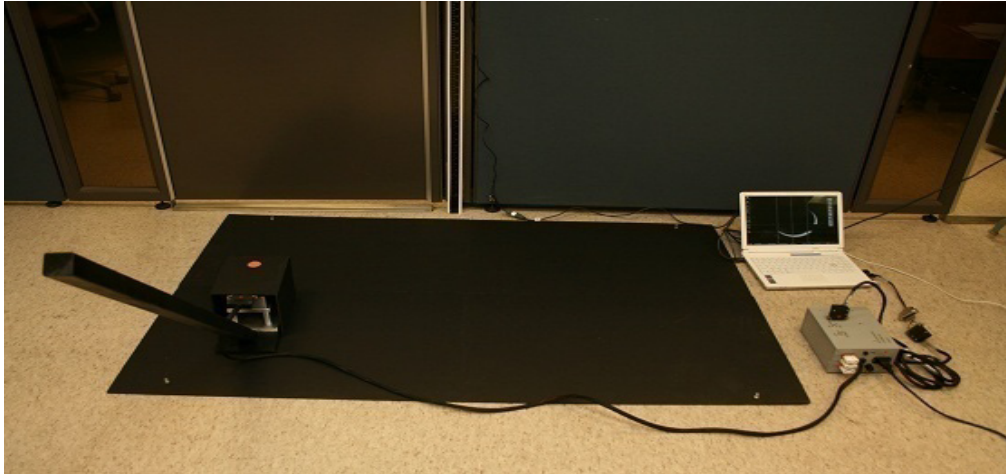
Figure B.1. Data collection system for Coarse and Fine alignment and calibration: Run-box, desktop, monitor and IMU on solid mount.
