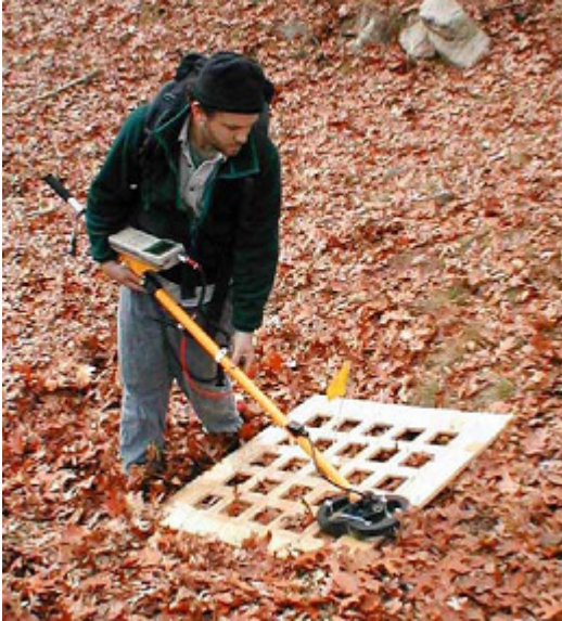
Figure 1.1. Collecting data on a grid over a suspected UXO (Bell and Collins, 2007)
