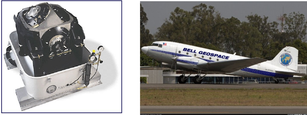
Figure 4.2: FTG gradiometer and aircraft (Bell Geospace, 2008)
